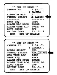
Select video/audio switching timing on SET UP MENU (REAL TIME or T-LAPSE).
