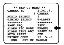
Select alarm recording mode on SET UP MENU (FRAME or SPOT.)
