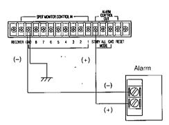
The polarities for the alarm and Alarm Control Output of the monitor should be matched.
