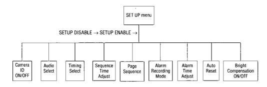
A set up operation can be performed with the following switches on the front panel.
