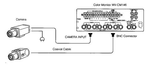
Connect single coaxial cables between the cameras and monitor (CAMERA INPUT). The maximum coaxial cable length is as follows;
