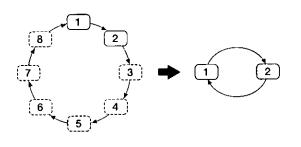
Note: In sequential switching the input connector, without connected cameras will be automatically skipped.
