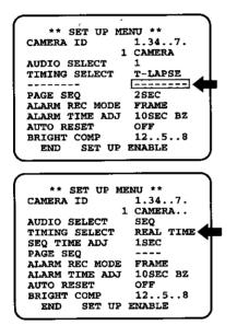
In case of T-LAPSE is selected for TIMING SELECT, sequential time synchronizes with the switching signal of the time lapse VCR. You cannot set by this monitor. In case of REAL TIME is selected for TIMING SELECT, you can select one of the two sequential time adjustments by MONITOR MODE switch;
