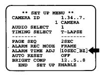
Set alarm (BZ) on or off with SET UP switch. When "BZ" is set on, adjust the alarm time on SET UP MENU.
