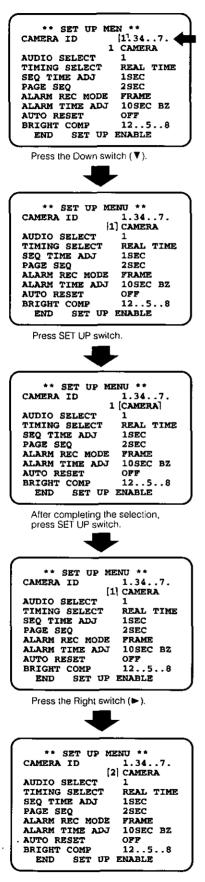
1-1. Move the cursor to "CAMERA ID," and select the desired camera using the Left (◄) or Right switch (►).
