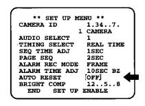
Set Automatic Reset On or Off on SET UP MENU (ON or OFF.)
