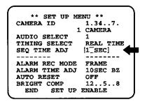
This menu appears only when REAL TIME is selected for TIMING SELECT while SEQ/QUAD is selected for MONITOR MODE.
